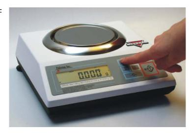
1. Place a container on the pan and tare it by pressing the "T" button.
