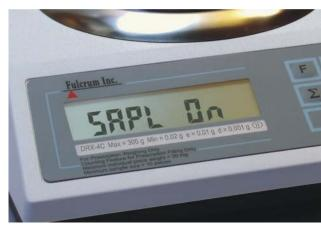
4. Press the T button to confirm and accept the sample weight.
